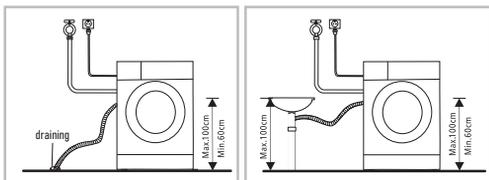
**NOTE:** If the free end of the hose is routed into a sink, use a special holding clamp (bracket) as in the case with a bathtub; secure the clamp with a chain or rope.
