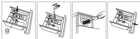
1. Press the latch (located above the rinser/conditioner compartment) and remove the tray.
