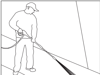
Figure 6 - Optimum angle to cleaning surface
