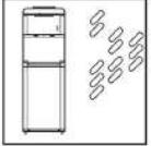
2. IT IS ALLOWED TO CONNECT THE DEVICE TO THE NETWORK ONLY AFTER FILLING ITS CONTAINERS WITH WATER. OPERATION OF THE DEVICE WITHOUT WATER IN CONTEINERS OR WITHOUT WATER IN A BOTTLE IS NOT ALLOWED.
